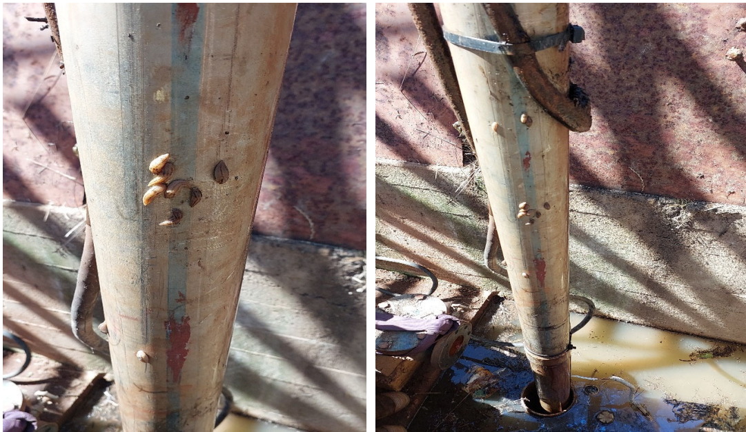
Condition of pumping equipment showing biological contamination.
