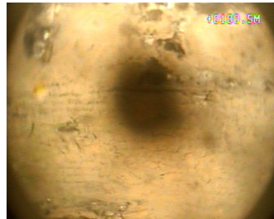
Threaded joints at 161.50m and 180.50m showing corrosion present.
